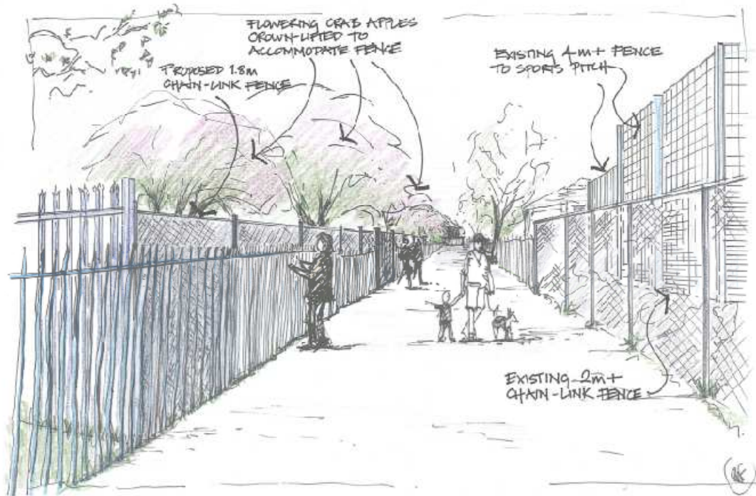
PROPOSED CHAIN LINK FENCE BEHIND RAILINGS ON ACCESS ROUTE FROM WOODSIDE AVENUE
